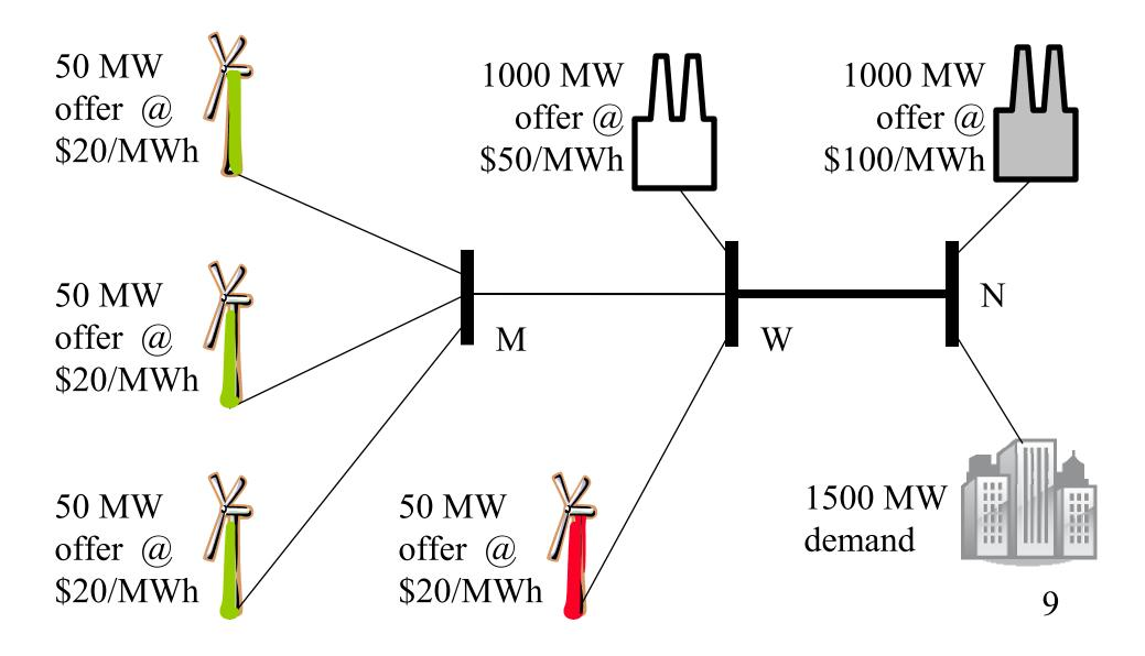
Dispatch for 1500 MW demand, unlimited transmission capacity.
