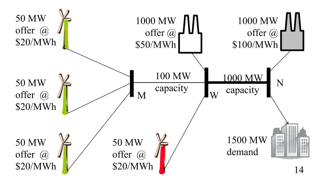
Dispatch for 1500 MW demand, limited transmission capacity.
