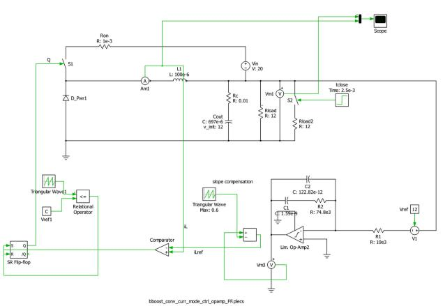
Experiment – 13: Peak Current Mode Control of Buck-Boost Converter with Slope Compensation
