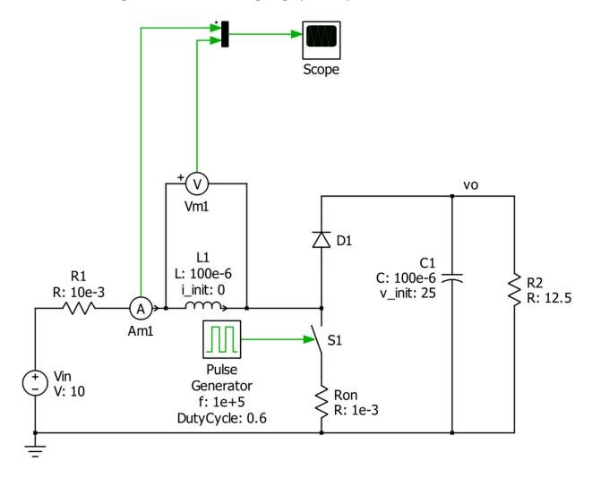
Experiment - 5: Step-Up (Boost) DC-DC Converter
