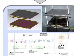
ORNL Coupling Coil Design based on first principles electro-magnetic design. System design tailored to minimize vehicle complexity, cost and packaging.
