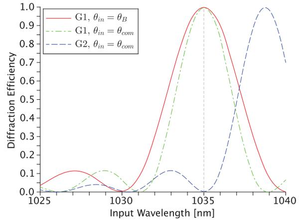
**Fig. 5.** Diffraction efficiency curves versus wavelength for two gratings, G1 and G2, in a sequential grating SBC system for the input angles corresponding to inputs A and B.
