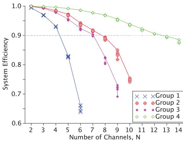
**Fig. 8.** Optimized multiplexed grating system efficiency for each of the four system parameter groups as a function of the number of channels in the system,  $N$ . Operating bandwidth is fixed at 1030–1040 nm. The dashed horizontal line indicates an arbitrary system efficiency goal of 90%. Stacked symbols indicate the results of repeated optimizer runs for a given set of inputs.
