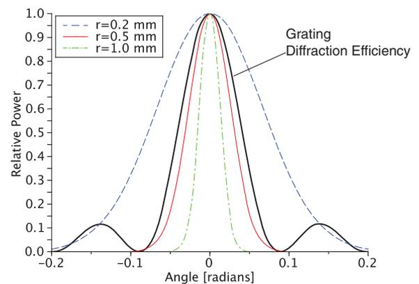
**Fig. 10.** Relative angular widths for Gaussian inputs at 1035 nm with various radii compared with the diffraction efficiency as a function of input angle (for a fixed wavelength) of a typical Group 1 grating centered at 1035 nm.
