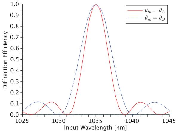
**Fig. 4.** Diffraction efficiency of a single volume Bragg grating as a function of wavelength for input angles corresponding to the two channels combined by this HOE. The grating parameters are described in the main text. Note how the horizontal scaling of the diffraction efficiency curve varies depending on which input angle is used.
