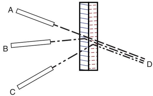
**Fig. 2.** Three-channel transmission-mode sandwiched grating SBC system utilizing two single-grating HOEs. Inputs A, B, and C operate at different wavelengths and are combined into output D. Ideally, input A is not diffracted by either grating, input B is strongly diffracted by the first grating and not diffracted by the second, and input C is strongly diffracted by the second grating and not diffracted by the first.
