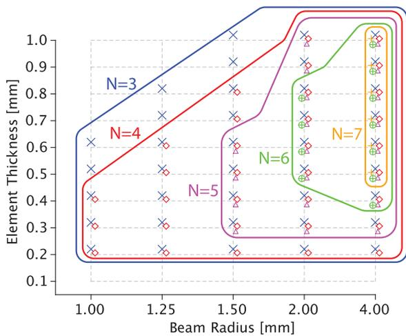
**Fig. 13.** Regions of beam radius ( $r$ ) and holographic element thickness ( $d$ ) where 90% system efficiency can be achieved in a multiplexed grating architecture for various numbers of channels  $N$ . The PSO optimizer was executed for combinations of thickness and radius at the intersections of the dashed lines, and the mark representing a particular number of channels is included at an intersection if the optimized system efficiency exceeded 90%.
