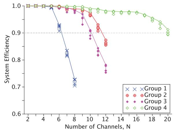
**Fig. 9.** Optimized cascaded grating system efficiency for each of the four system parameter groups as a function of the number of channels in the system,  $N$ . Operating bandwidth is fixed at 1030–1040 nm. The dashed horizontal line indicates an arbitrary system efficiency goal of 90%. Stacked symbols indicate the results of repeated optimizer runs for a given set of inputs.
