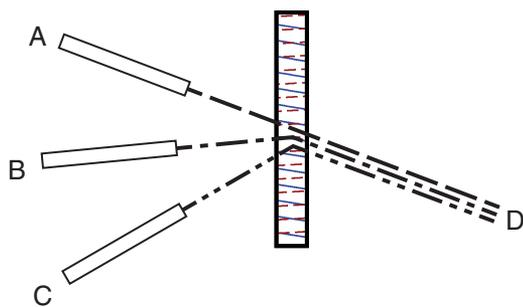
**Fig. 3.** Ideal three-channel transmission-mode multiplexed grating SBC system utilizing a dual-grating HOE. Inputs A, B, and C operate at different wavelengths and are combined into output D. Ideally, input A is not diffracted by either grating and inputs B and C are each strongly diffracted by one of the multiplexed gratings but not the other.
