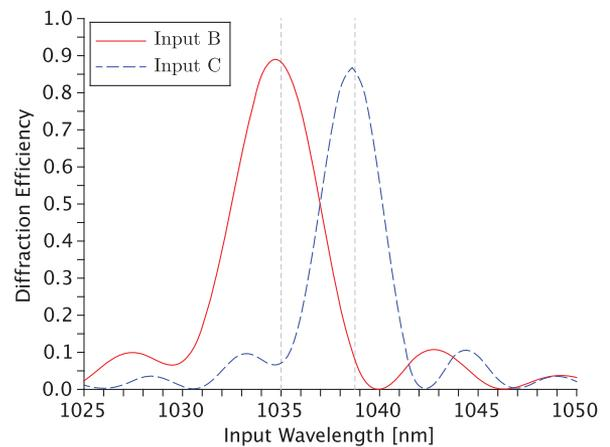
**Fig. 6.** Diffraction efficiencies at the system output for inputs B and C of a two-grating multiplexed SBC system formed by trivially collapsing the two gratings of a sandwiched grating system into a single HOE.
