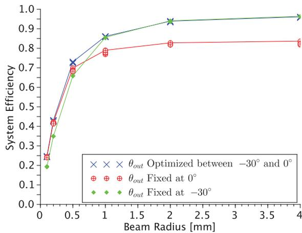
**Fig. 11.** Efficiency of a five-channel multiplexed grating system as a function of input beam radius. The material thickness is kept constant at 0.5 mm. The three curves indicate the efficiency results with the system output angle fixed at  $0^\circ$  (Group 1), fixed at  $-30^\circ$  (Group 2), and optimized between those two angles. Stacked symbols indicate the results of repeated optimizer runs.
