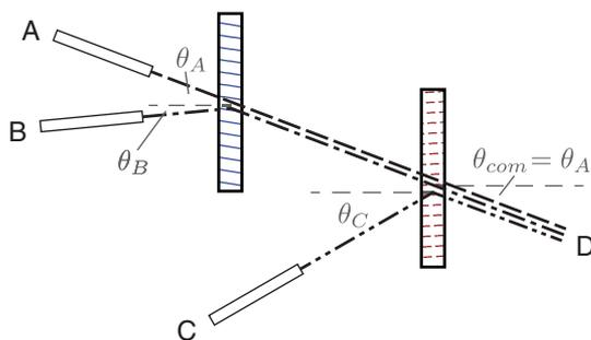
**Fig. 1.** Three-channel transmission-mode cascaded grating SBC system utilizing two single-grating HOEs. Inputs A, B, and C operate at different wavelengths and enter the system at angles  $\theta_A$ ,  $\theta_B$ , and  $\theta_C$ , respectively. These inputs are combined into output D, which leaves the system at angle  $\theta_{com} = \theta_A$ .
