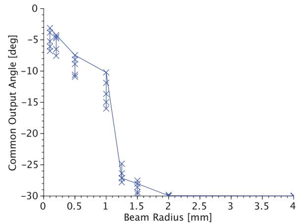
**Fig. 12.** Optimized output angle for a five-channel multiplexed grating system as a function of input beam radius. The material thickness is kept constant at 0.5 mm. Stacked symbols indicate the results of repeated optimizer runs, and the solid line indicates the angles associated with the highest achieved system efficiency (see Fig. 11) for a given input beam radius.
