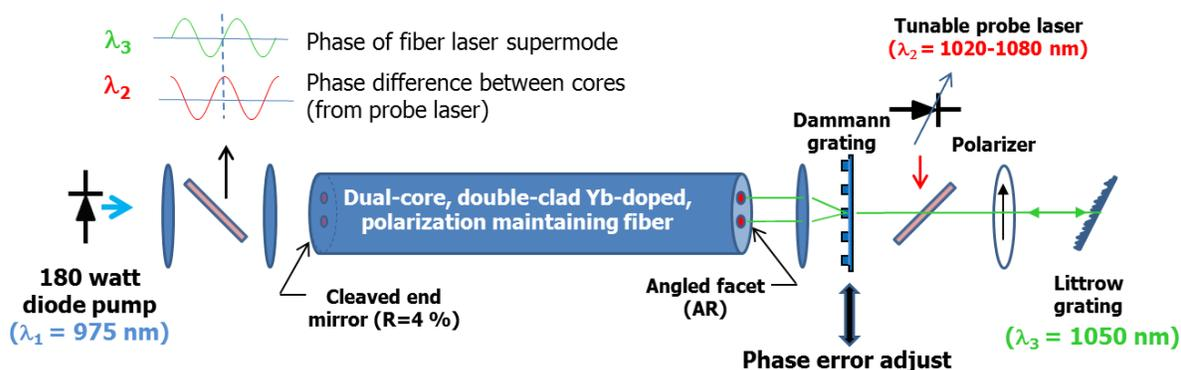
Fig. 1. Experimental set-up for measuring the effects of nonlinearities on a coherently combined laser using a Damann grating cavity.
