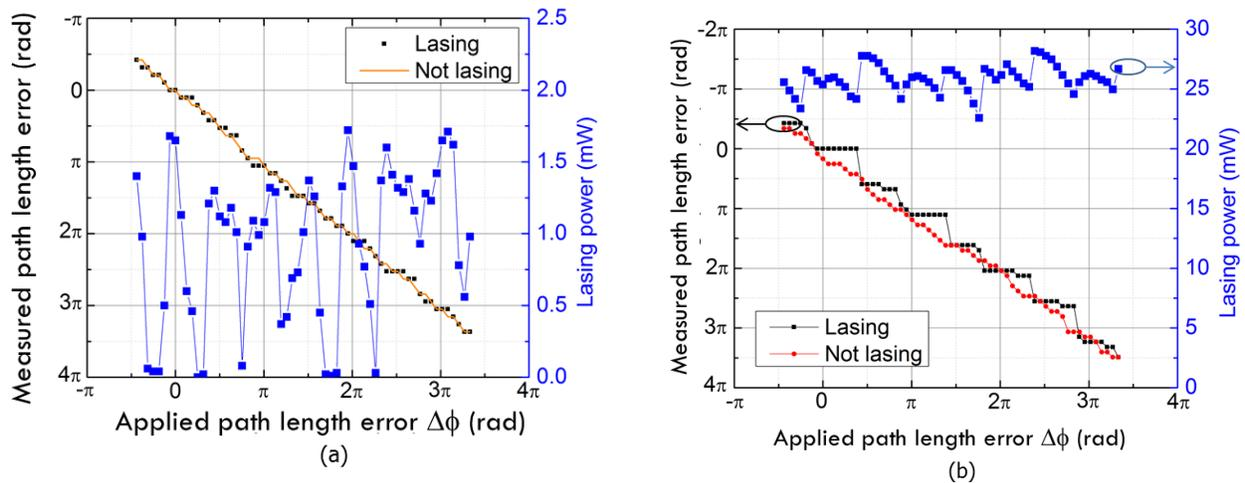
Fig. 2. Measurements of laser power (right axis) and differential path length errors (left axis) for lasers coherently combined in a Damman grating cavity as a function of path length error. a) 1.2 watts of pump power, b) 2.4 watts of pump power.
