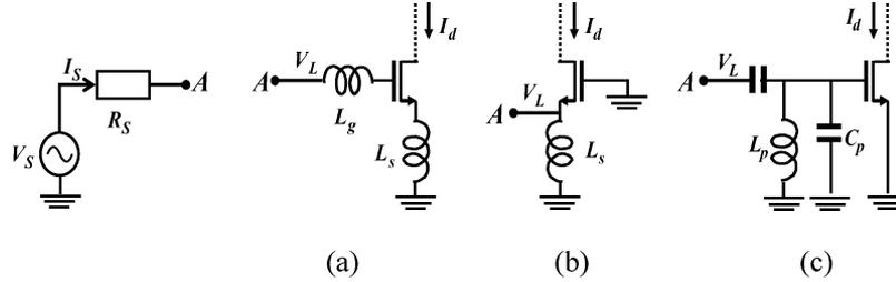
Fig. 13. LNA input matching. (a) CS-LNA with a source-degeneration inductor. (b) CG-LNA. (c) CS-LNA with a shunt inductor.
