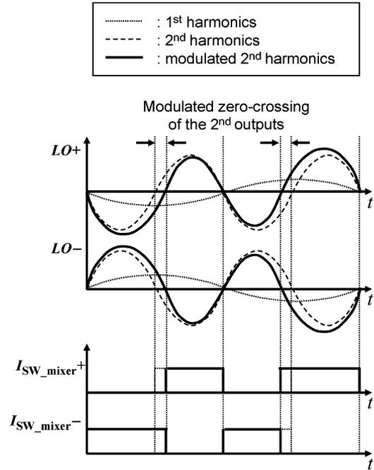
Fig. 7. Modulated second harmonics and switching currents by first harmonics.
