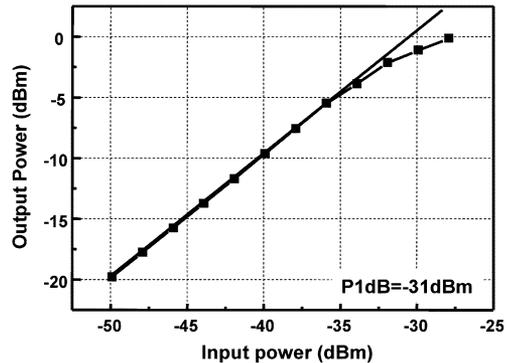
Fig. 21. Output power versus input power of the proposed front-end.
