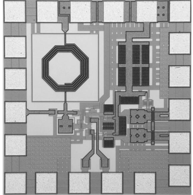
Fig. 17. Microphotograph of a conventional merged LNA and SB mixer (occupies an area of  $0.85 \times 0.9 \text{ mm}^2$ ).
