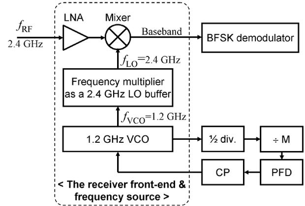
Fig. 1. Receiver architecture suitable for a low-power application. (The dotted line indicates the boundary of the fabricated chip.)
