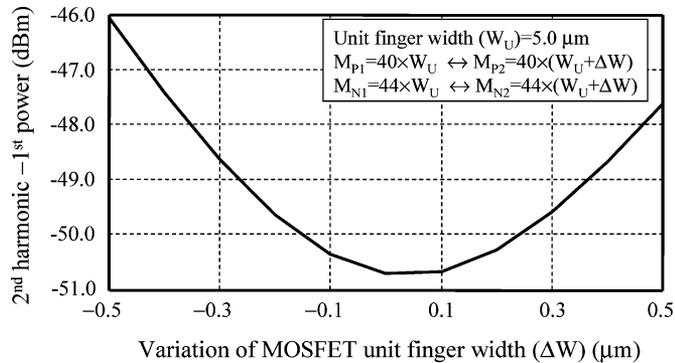
Fig. 9. Device width mismatch versus first harmonic cancellation effect.
