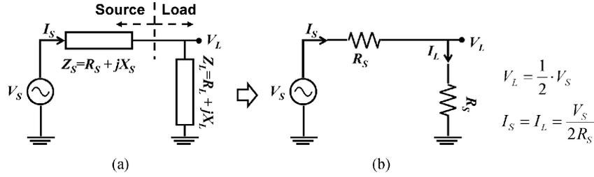
Fig. 12. Simplified matching circuit for voltage and current.
