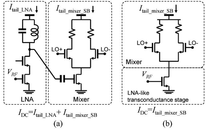
Fig. 10. Conventional front-end configurations. (a) A cascade of LNA and SB mixer. (b) Merged LNA and SB mixer.
