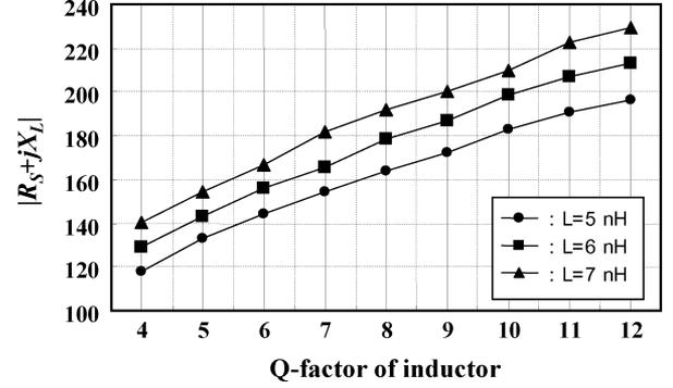
Fig. 15. Q-factor versus input impedance of matching circuit.
