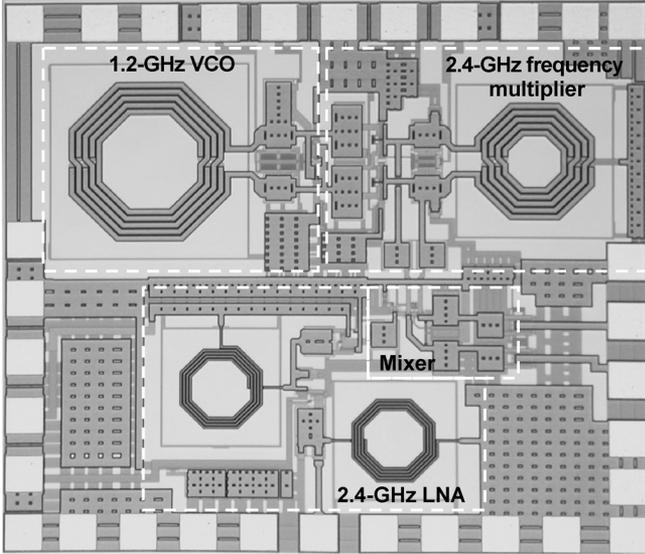
Fig. 16. Fabricated current-reused folded-cascode receiver front-end and LO source ( $1.6 \times 1.45 \text{ mm}^2$  including pads).
