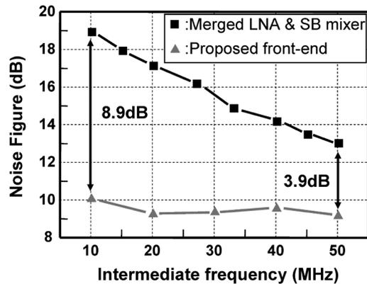
Fig. 20. Measured SSB NF of fabricated front-ends.
