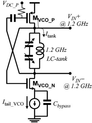
Fig. 2. Circuit implementation of a 1.2-GHz VCO ( $M_{VCO\_P} = 225/0.18 \mu\text{m}$ ,  $M_{VCO\_N} = 225/0.18 \mu\text{m}$ ,  $L = 12 \text{ nH}$ ).
