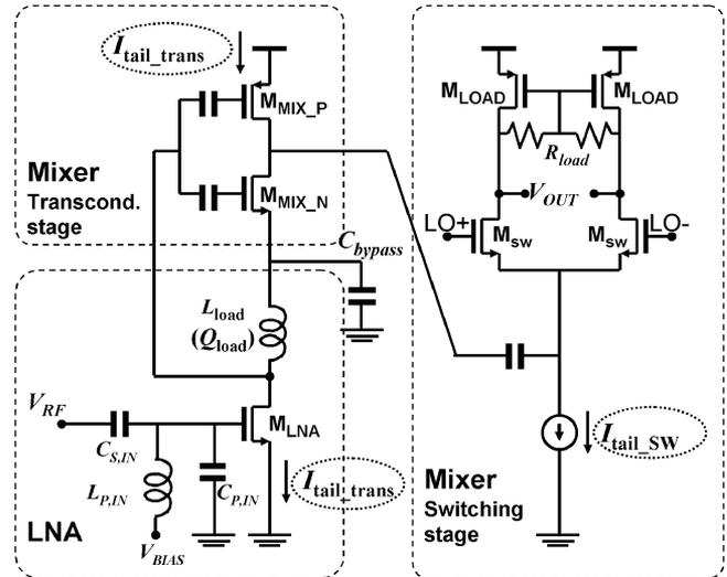
Fig. 11. Proposed current-reused folded-cascode front-end ( $M_{LNA} = 75/0.18 \mu\text{m}$ ,  $M_{MIX\_N} = 40/0.18 \mu\text{m}$ ,  $M_{MIX\_P} = 195/0.18 \mu\text{m}$ ,  $M_{SW} = 35/0.18 \mu\text{m}$ ,  $M_{LOAD} = 480/0.5 \mu\text{m}$ ,  $R_{load} = 20 \text{ k}\Omega$ ,  $L_{load} = 4.5 \text{ nH}$ ,  $L_{P,IN} = 6.3 \text{ nH}$ ).
