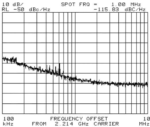
Fig. 18. Measured phase noise of the fabricated frequency source.
