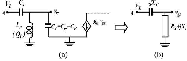
Fig. 14. CS-LNA with a shunt inductor. (a) Equivalent circuit. (b) Matching condition.
