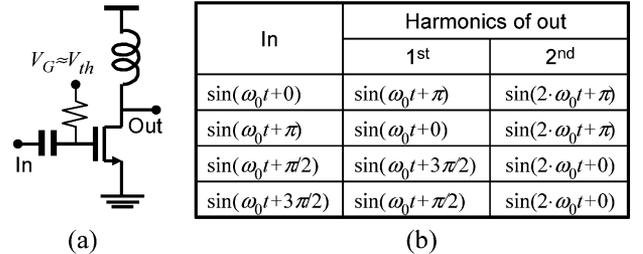
Fig. 4. (a) nMOS pinch-off clipper. (b) Phase of first and second harmonic output signals according to input signals.
