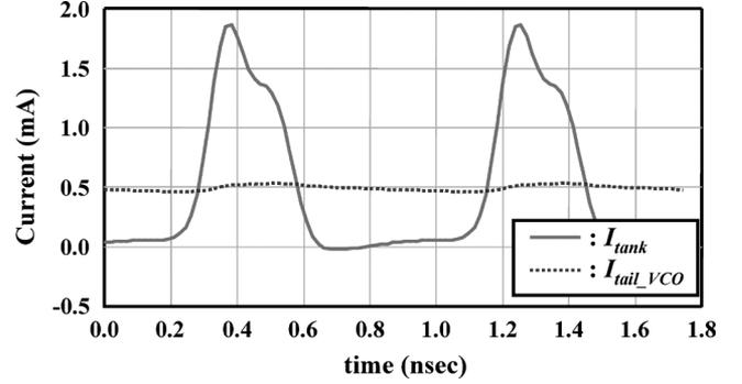
Fig. 3. Simulation result of the proposed VCO.
