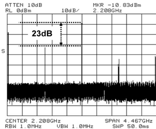
Fig. 19. Measured output spectrum of the frequency source at the center frequency of 2.21 GHz.
