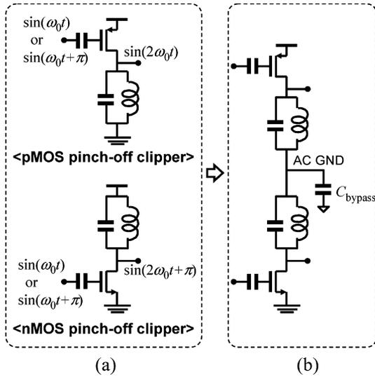
Fig. 5. Concepts of the proposed frequency multiplier. (a) Phase of second harmonics of nMOS and pMOS pinch-off clippers. (b) Current-reused frequency multiplier for power reduction.
