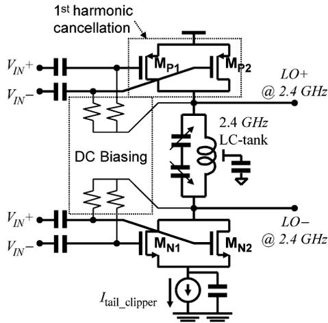
Fig. 6. Circuit topology of the proposed 2.4-GHz current-reused differential frequency multiplier ( $M_{P1} = M_{P2} = 200/0.18 \mu\text{m}$ ,  $M_{N1} = M_{N2} = 220/0.18 \mu\text{m}$ ,  $L = 7 \text{ nH}$ ).
