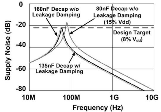
**Fig. 8: Frequency diagram of supply noise w/ and w/o considering the leakage damping effects for decap assignment.**
