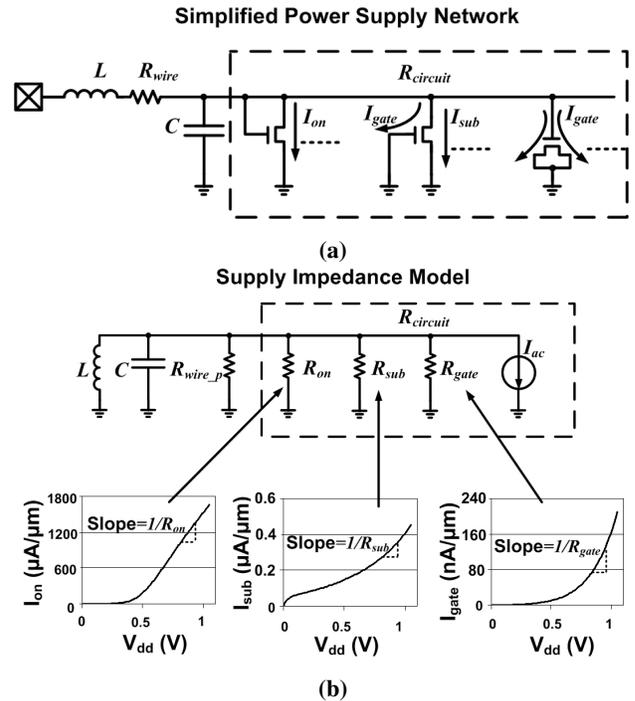
Fig. 2: (a) Simplified power supply model used in this paper; (b) Supply impedance model including the resistance of the circuit itself. Each current component has different damping effects due to the difference in equivalent resistance.
