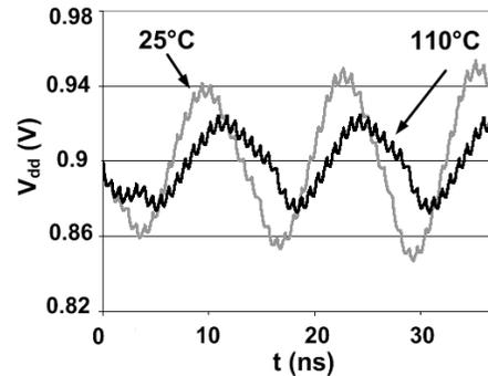
Fig. 6: Simulated noise waveforms at 25°C and 110°C for ISCAS benchmark circuits.
