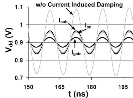
**Fig. 4: Supply resonant noise damped by different current components. Gate leakage provides largest damping effect for the same amount of current.**
