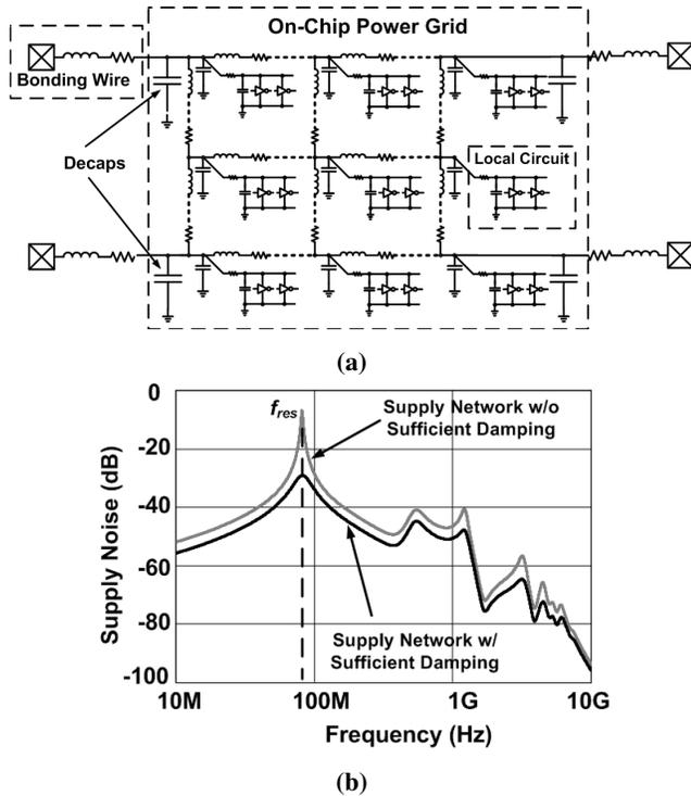
Fig. 1: (a) Model of power supply mesh; (b) Simulated frequency spectrum of supply noise from the model in (a).
