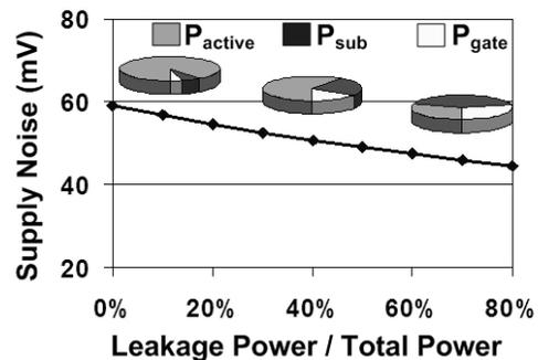
Fig. 7: Resonant supply noise versus leakage power ratio.
