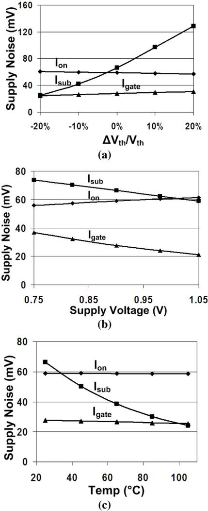
Fig. 5: Simulated damping effects under PVT variation. (a) Threshold voltage variation; (b) Supply voltage variation; (c) Temperature variation. Note that larger damping effect leads to smaller supply noise.
