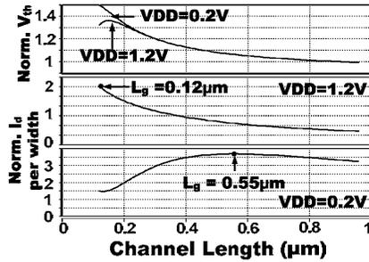
Fig. 3. Dependency of normalized  $V_{th}$  and current-per-width on channel length
