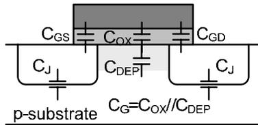
Fig. 4. Capacitance in subthreshold MOS device
