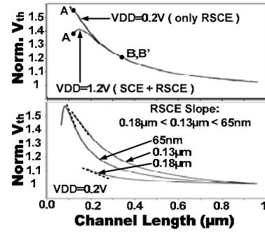
Fig. 1. Dependency of normalized  $V_{th}$  on channel length for VDD=1.2V and 0.2V
