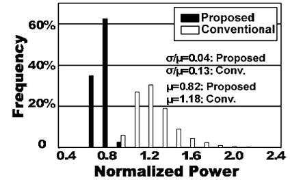
Fig. 7. Power distribution comparison for a static inverter.
