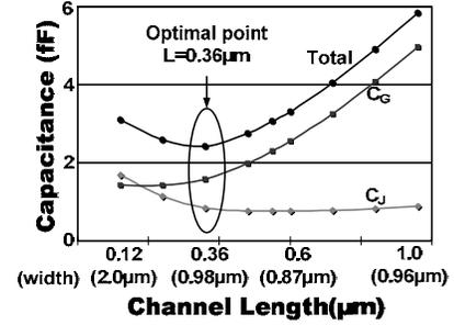
Fig. 5. Capacitance vs. channel length for constant current
