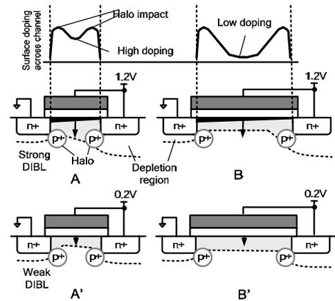
Fig. 2. Device cross sections corresponding to A, A', B, and B' in Fig. 1. Surface doping across channel is shown to illustrate the RSCE.
