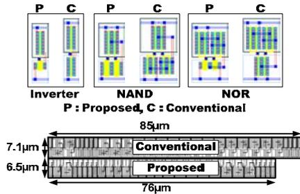
Fig. 8. Layout comparison for basic logic gates and sample delay chain.
