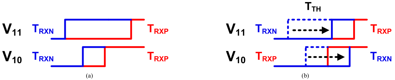
Fig. 8. Example of how tunable delay used to produce different threshold. (a) Timing diagram before the tunable delay. (b) After the delay, both two edge delay T_{TH} . The threshold delay is align to middle of T_{RXN} and T_{RXP} .
