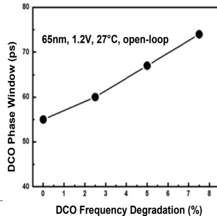
Fig. 6. (Upper) Measured open-loop DCO phase window before and after stress. (Lower) Measured open-loop phase window versus open-loop DCO frequency degradation.
