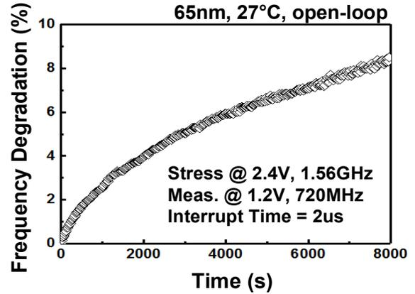
Fig. 5. Measured frequency degradation of open-loop DCO using beat frequency detection circuit.
