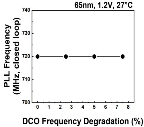
Fig. 9. Closed-loop PLL frequency remains constant despite DCO frequency degradation.
