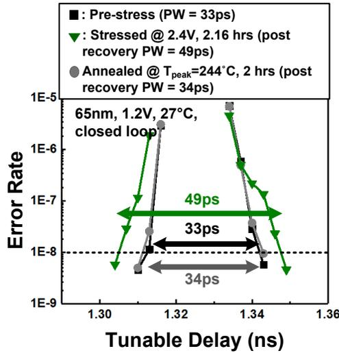
Fig. 11. Measured closed-loop phase window curves for pre-stress, stressed, and annealed DCOs.
