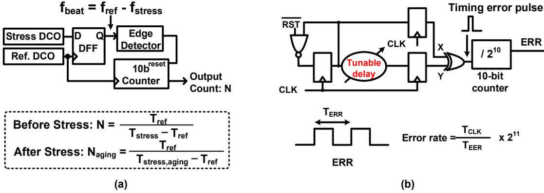
Fig. 3. (a) Frequency degradation monitor based on “silicon odometer” beat frequency detection scheme. (b) Phase window monitor based on a tunable delay.
