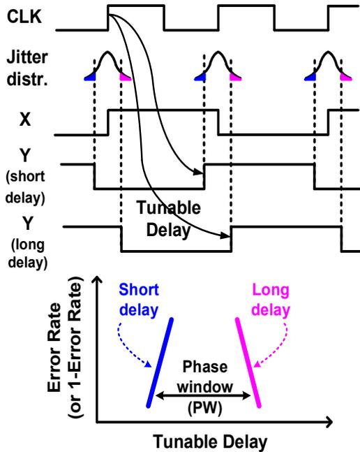
Fig. 4. Phase noise degradation can be indirectly measured by sweeping the tunable delay.
