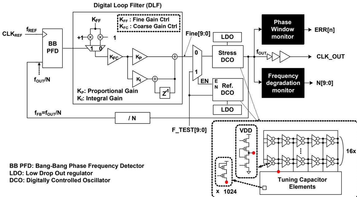
Fig. 1. All-digital PLL with on-chip frequency and phase noise measurements circuits.
