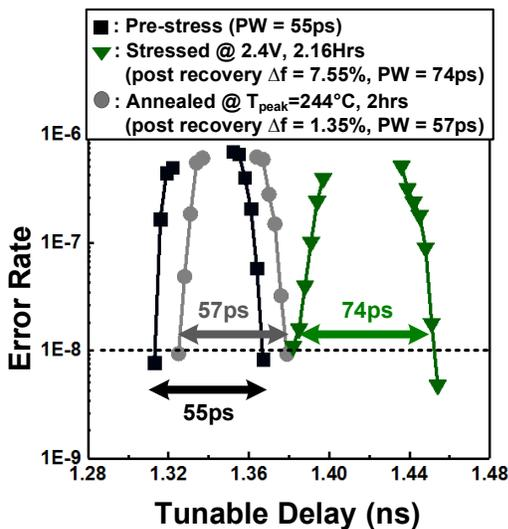
Fig. 8. Measured open-loop phase window curves for pre-stress, stressed, and annealed DCOs.
