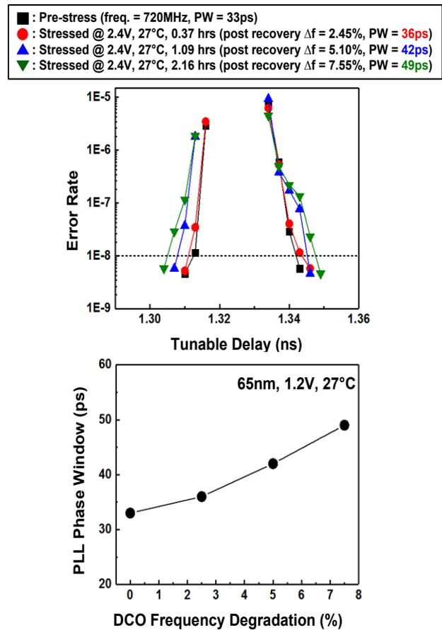
Fig. 10. Measured PLL phase window before and after stress.
