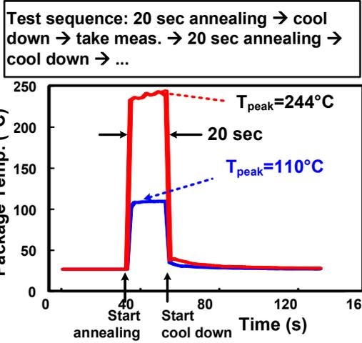
Fig. 7. (Upper) Measured frequency shift under different stress and recovery conditions. (Lower) Annealing test sequence. The package is cooled down after each 20 second annealing period to ensure accurate frequency measurements.
