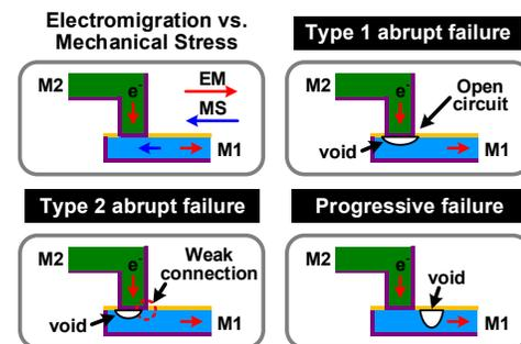
Fig. 10. Void location of different failure types.
