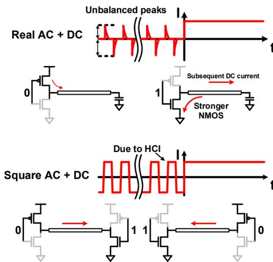
Fig. 19. Mismatch in forward and backward peak currents during real AC stress may result in a longer lifetime in subsequent DC stress.
