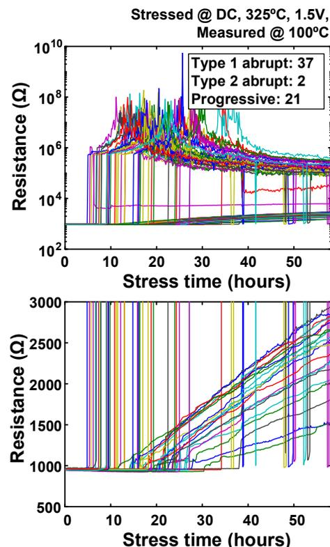
Fig. 8. Resistance traces under DC stress.
