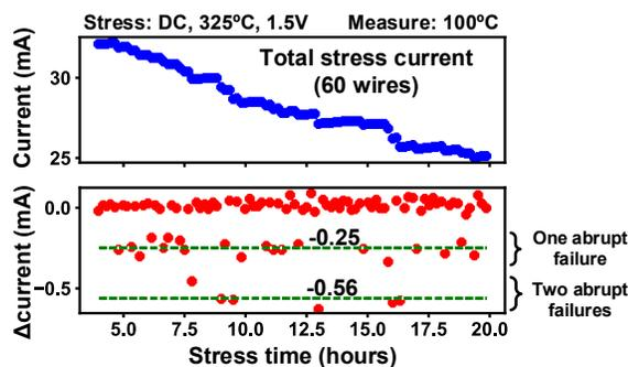
Fig. 11. (Above) Total stress current versus stress time. (Below) The change in the stress current in each 10 minutes stress interval indicating the number of EM failures and the stress current of each DUT.
