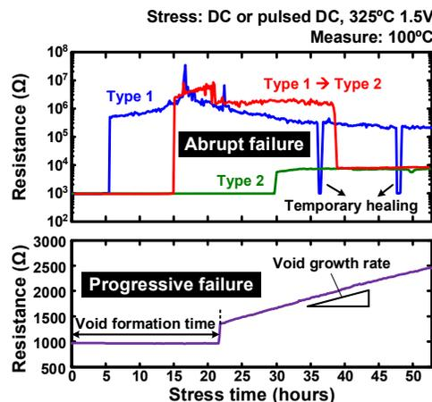
Fig. 9. Resistance trace samples showing abrupt and progressive failures.
