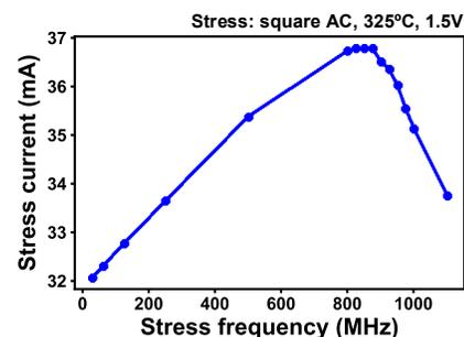
Fig. 12. Total stress current versus stress frequency for square AC stress. Stress current decreases beyond 900 MHz due to signal swing degradation so we chose 900 MHz as the maximum stress frequency.
