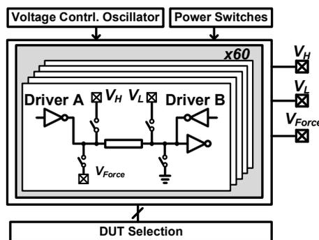
Fig. 2. EM test array with 60 DUT wires.
