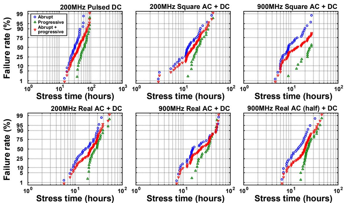
Fig. 22. Abrupt, progressive, and total failure distributions under various stress modes.
