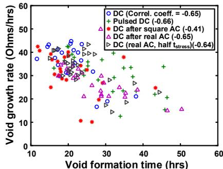
Fig. 14. Correlation between void formation time and void growth rate for progressive failures.
