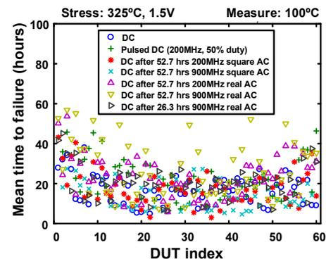
Fig. 21. MTF versus DUT location. DUTs located in the center of the heating area show a marginally shorter MTF. This can be attributed to a subtle temperature gradient within the heating area.
