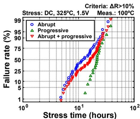
Fig. 23. Abrupt failure and progressive failure distributions for DC stress, along with the combined distribution. The individual distributions follow a lognormal distribution.
