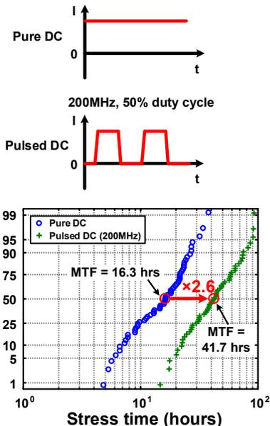
Fig. 15. Failure time comparison between DC and pulsed DC.
