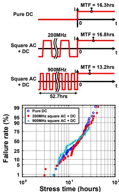
Fig. 17. Failure time comparison between DC and square AC + DC.
