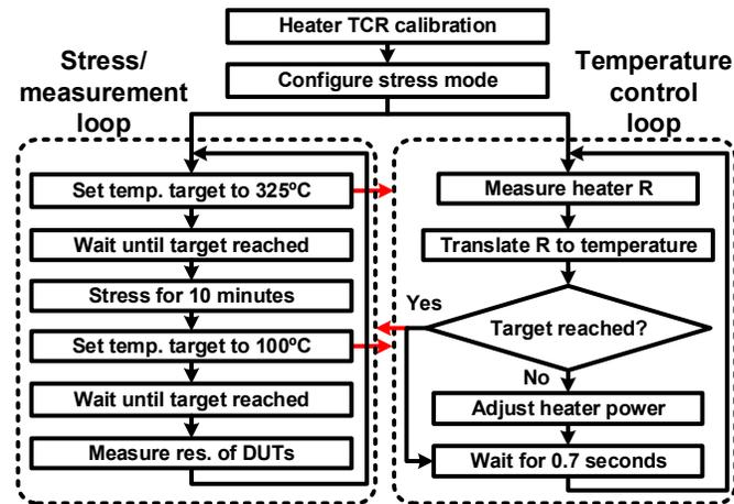
Fig. 7. Script based automated test flow. Two control loops (stress/measurement and temperature control) were implemented.
