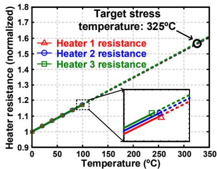
Fig. 4. Temperature Coefficient of Resistance (TCR) measurements from 3 heater leads and temperature extrapolation method.
