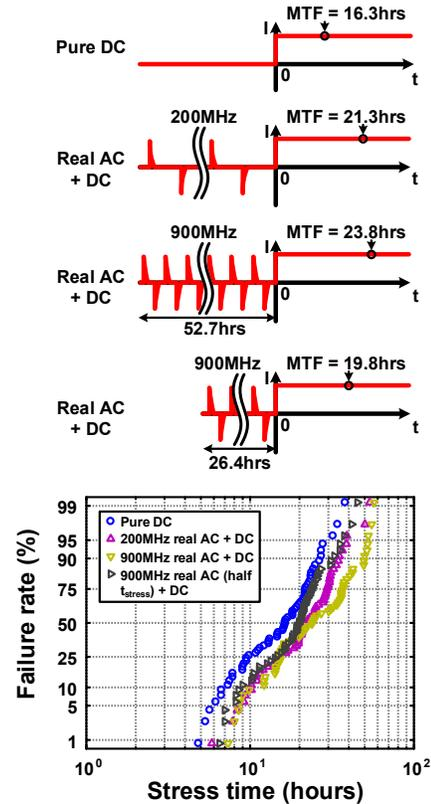
Fig. 18. Failure time comparison between DC and real AC + DC.
