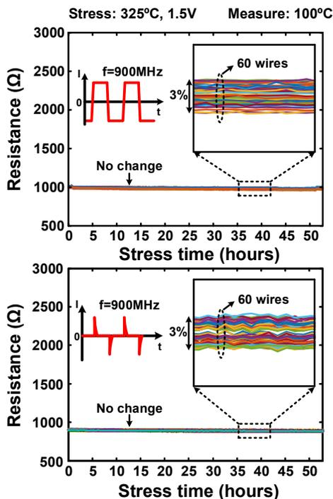
Fig. 13. Resistance traces under square AC and real AC stress modes at 900 MHz.
