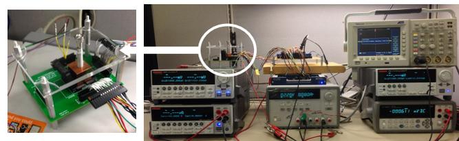
Fig. 6. 32 nm EM test chip measurement setup.
