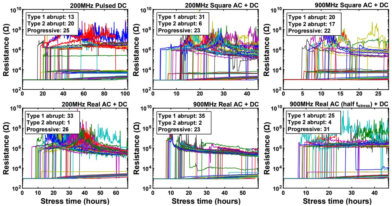
Fig. 16. Resistance traces and failure type ratios under various stress modes.
