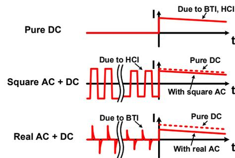
Fig. 20. Transistor aging during pre-stress may reduce the stress current in subsequent DC stress.
