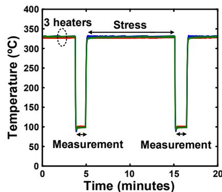
Fig. 5. Temperature cycling for stress and measurement modes. The DUT temperature was lowered from 325 °C to 100 °C during resistance measurements to suppress leakage current in the selection switches.
