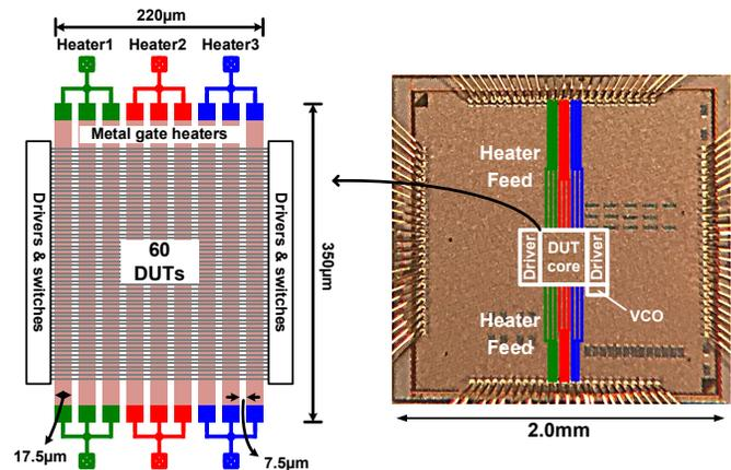
Fig. 3. (Left) Vertical metal gate heaters placed underneath 60 horizontal EM wires. (Right) Die photo of the 32nm EM test chip.
