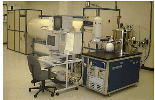
Fig. 5. Particle accelerator used for radiation testing (Source: University of Minnesota Characterization Facility)
