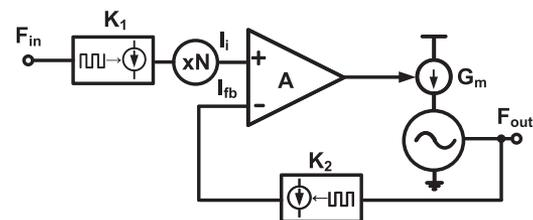
Fig. 1. Proposed frequency synthesizers based on current multiplier.
