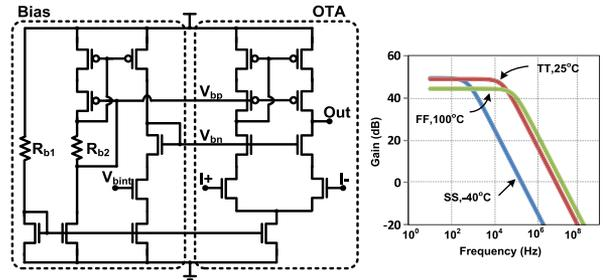
Fig. 4. High-gain OTA schematic and simulated gain plot.
