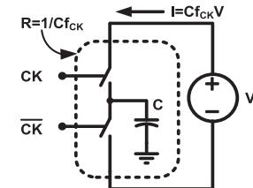
Fig. 3. Frequency-to-current conversion circuit.
