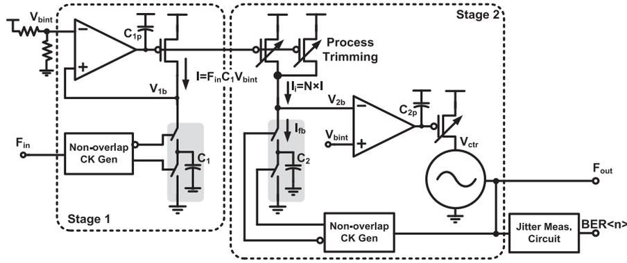
Fig. 2. Proposed current multiplier-based frequency synthesizer schematic with on-chip periodic jitter measurement circuit.
