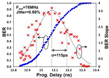
Fig. 13. BER and periodic jitter from on-chip jitter measurement block.
