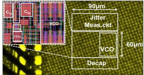
Fig. 10. 32-nm test chip die photograph and core layout.
