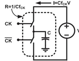
Fig. 3. Frequency-to-current conversion circuit.
