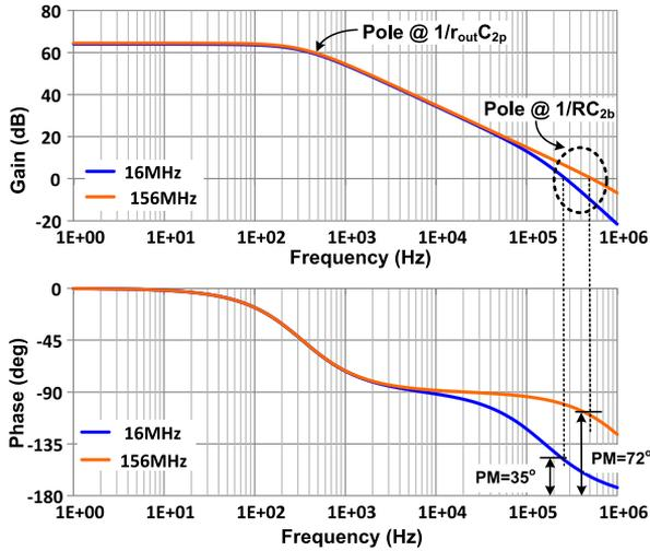
Fig. 7. AC simulation plot of loop model.
