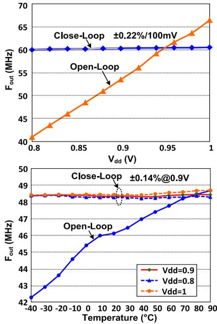
Fig. 12. Measured voltage and temperature dependence.
