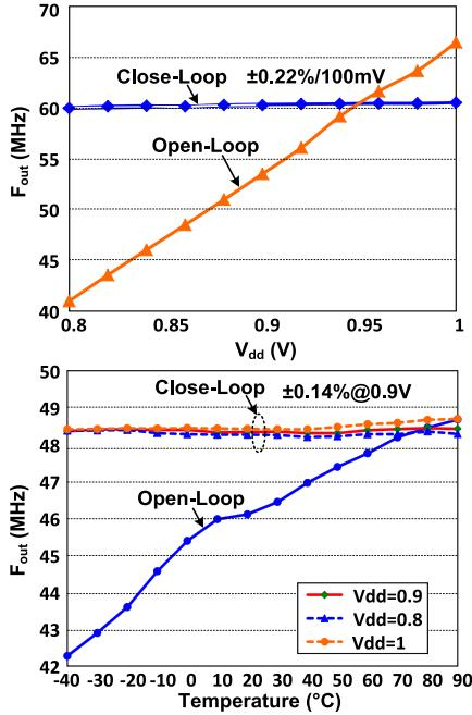
Fig. 12. Measured voltage and temperature dependence.
