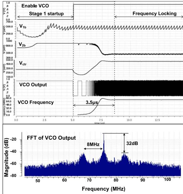
Fig. 8. Frequency synthesizer transient response and output fast Fourier transform (FFT) (simulation).
