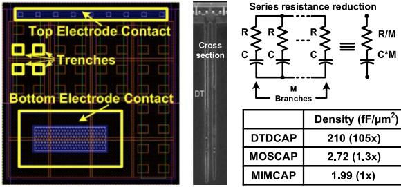
Fig. 5. Deep trench capacitor for area reduction.
