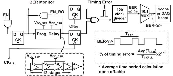
Fig. 9. On-chip periodic jitter measurement circuit [11].
