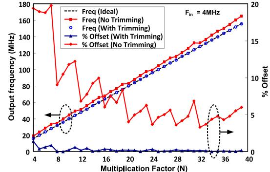
Fig. 11. Process trimming results.
