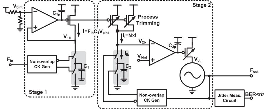
Fig. 2. Proposed current multiplier-based frequency synthesizer schematic with on-chip periodic jitter measurement circuit.
