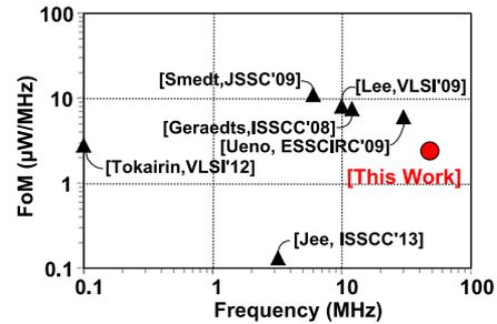
Fig. 14. FoM comparison with other clock generators.
