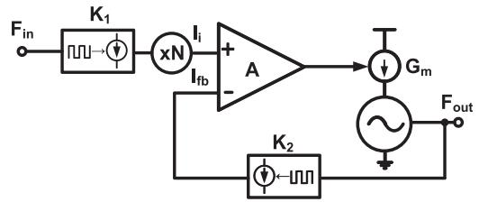
Fig. 1. Proposed frequency synthesizers based on current multiplier.
