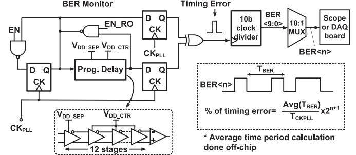
Fig. 9. On-chip periodic jitter measurement circuit [11].
