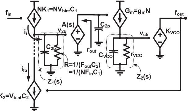
Fig. 6. Equivalent small signal model for loop stability analysis.
