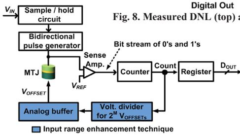
Fig. 10. Block diagram of MTJ-based ADC with input range expanding circuits. A voltage divider and an analog buffer control the MTJ bottom node voltage.
