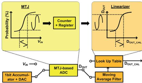
Fig. 7. Compensating for MTJ non-linearity using digital calibration [5, 6].
