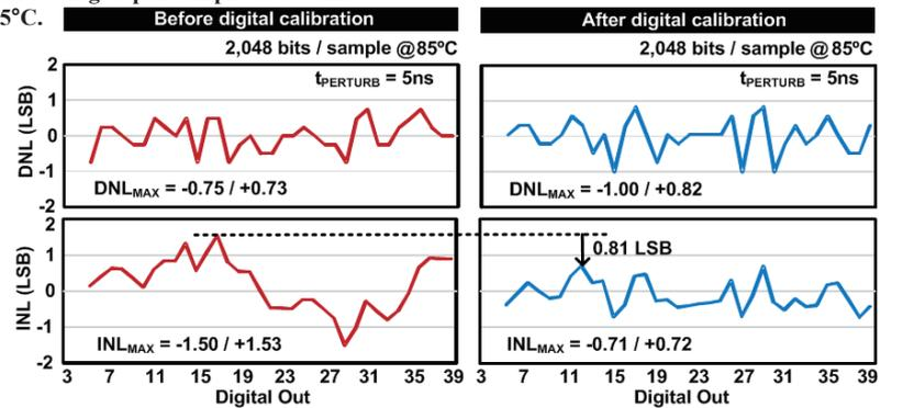
Fig. 8. Measured DNL (top) and INL (bottom) before and after digital calibration.
