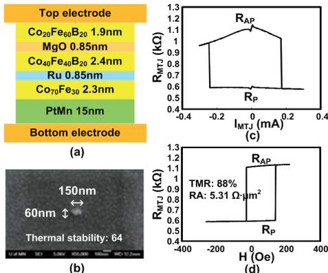
Fig. 1. CoFeB/MgO MTJ used in our experiments. (a) Vertical structure, (b) SEM image, (c) R-I, and (d) R-H hysteresis curves.
