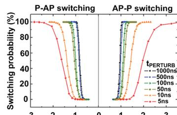
Fig. 2. Measured MTJ switching probability versus applied voltage [2].
