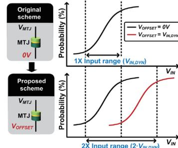
Fig. 9. Illustration of proposed input range enhancement technique.
