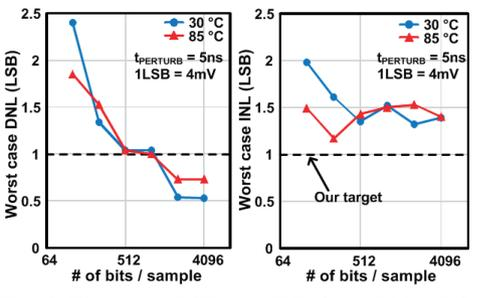
Fig. 6. Worst case DNL and INL for a 5-bit ADC resolution (i.e., 1 LSB=4mV) measured under two different temperatures (30, 85°C).
