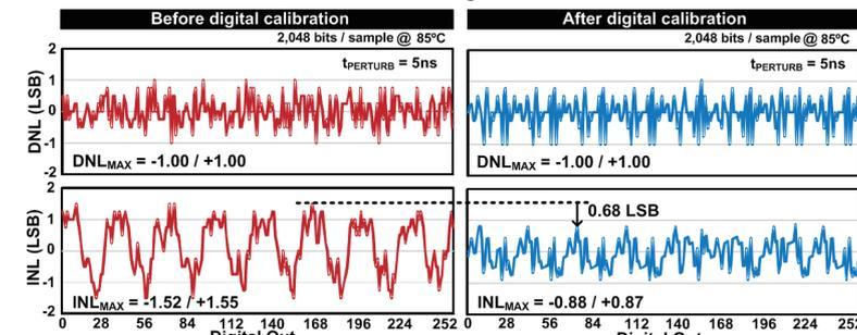
Fig. 12. Measured DNL (top) and INL (bottom) before and after digital calibration using the proposed input range enhancement technique.
