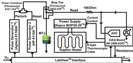
Fig. 4. MTJ-based ADC measurement setup with 1mV voltage resolution and <1°C temperature accuracy.
