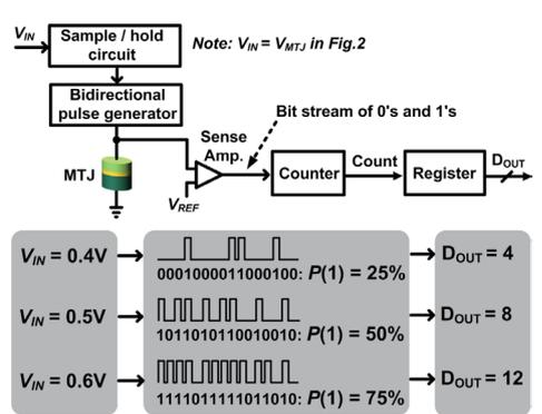
Fig. 3. Block diagram and operating principle of the proposed MTJ-based ADC.
