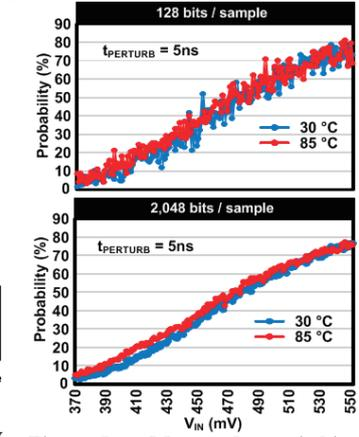
Fig. 5. Measured switching probability curve for 128 and 2,048 bits averaged per sample at 30 and 85°C.
