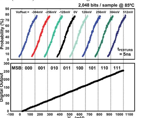
Fig. 11. Measured probability and corresponding digital output achieving an 8x wider input voltage range.
