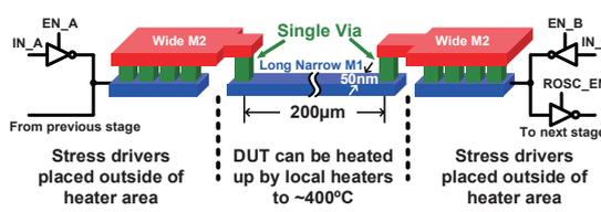
Fig. 2. EM DUT used in our experiment. Stress current is applied to a minimum width M1 wire with single via placed on both sides.
