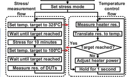
Fig. 6. Software flow for automatic EM measurements and temperature control.
