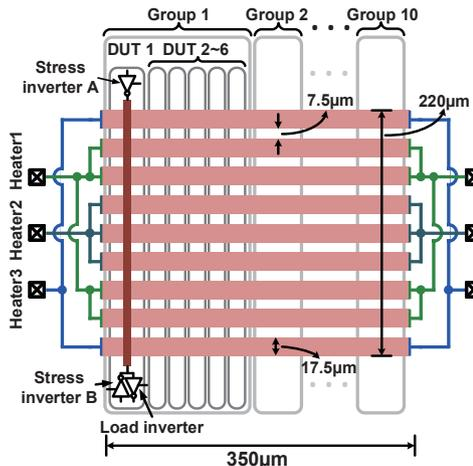
Fig. 4. Test chip floorplan showing 3 individually-controlled local heaters and 6x10 EM metal wires.
