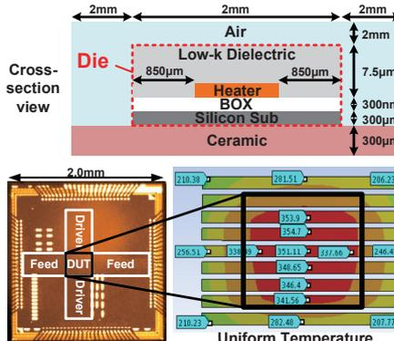
Fig. 5. Die photo and temperature sim. results.
