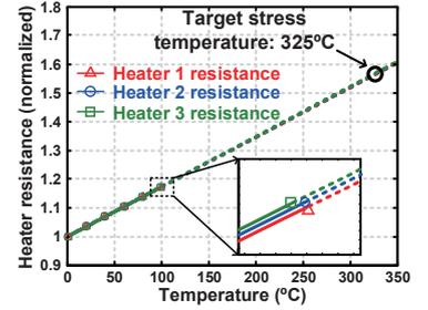
Fig. 3. Temperature coefficient of resistance (TCR) measured from actual test chip.
