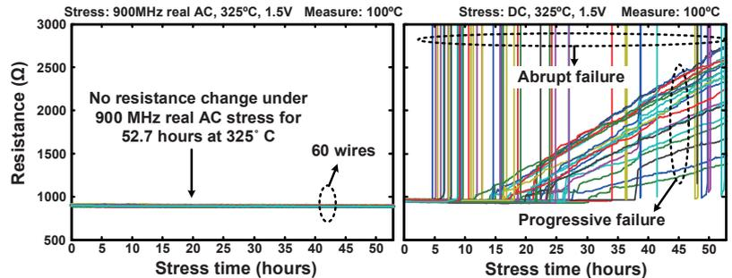
Fig. 8. Resistances traces under real AC (left, 900MHz) and DC (right) stress.
