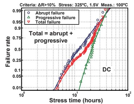
Fig. 10. Abrupt and progressive failure EM statistics under DC stress.
