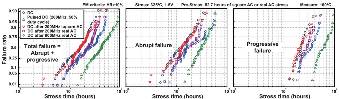
Fig. 11. Comparison between DC, pulsed DC (200MHz), DC after square AC (200MHz) and DC after real AC (200MHz and 900MHz). AC stress was applied for 52.7 hours. Time-to-failure distributions for combined (left), abrupt (middle) and progressive (right) failures.
