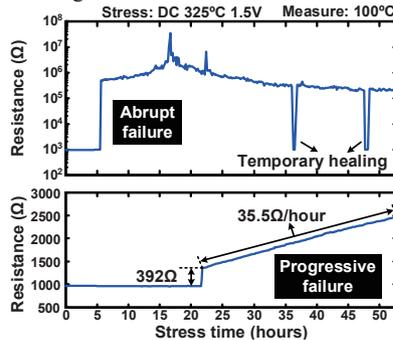
Fig. 9. Abrupt and progressive failure resistance traces measured from chip.
