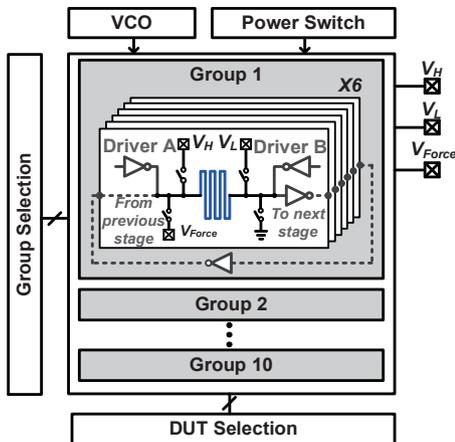
Fig. 7. Full chip schematic showing 4-terminal Kelvin resistance measurement circuit.
