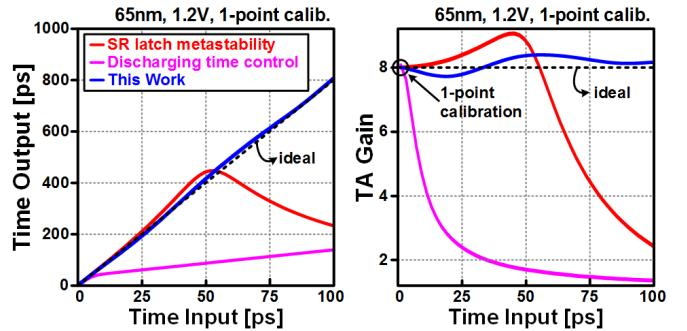
Fig. 4. Simulated time amplifier output and gain for  $N=7$  (i.e. 8x time amplifier) with 1-point calibration.
