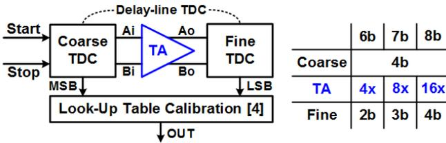
Fig.6. Two-step TDC circuit block diagram.
