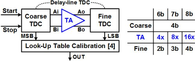
Fig.6. Two-step TDC circuit block diagram.
