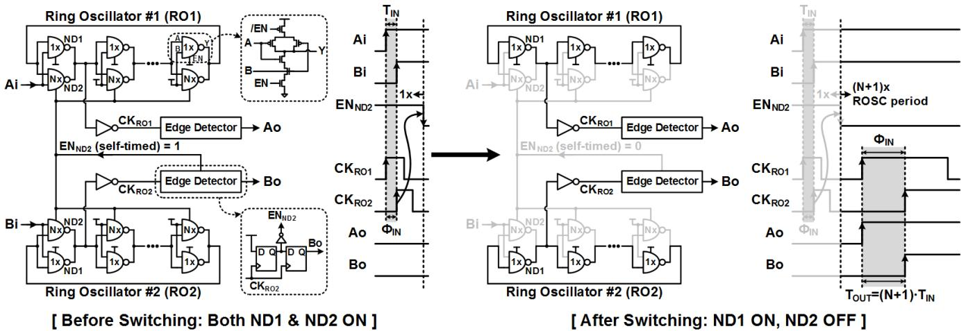
Fig.1. Proposed switched ring-oscillator based time amplifier circuit and its timing diagram before/after the switching operation.
