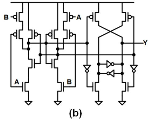
Fig.7. (a) 4bit coarse delay line TDC circuit. A reconfigurable 2/3/4bit Fine TDC has the same circuitry while having 1/2/4 DL stages. (b) Arbiter circuit [5].
