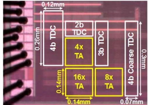
Fig.11. Chip micrograph.
