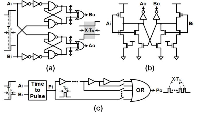
Fig.3. Existing time amplifier circuits based on (a) SR-latch metastability [1], (b) discharging time control [2] and (c) pulse-train [3]
