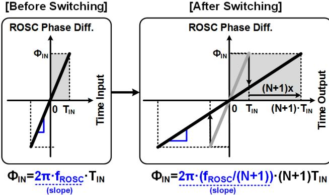
Fig. 2. Switched ring-oscillator based time amplifier mechanism.
