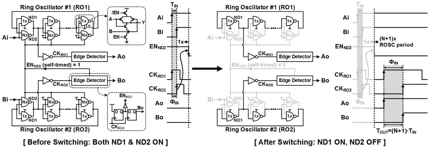
Fig.1. Proposed switched ring-oscillator based time amplifier circuit and its timing diagram before/after the switching operation.
