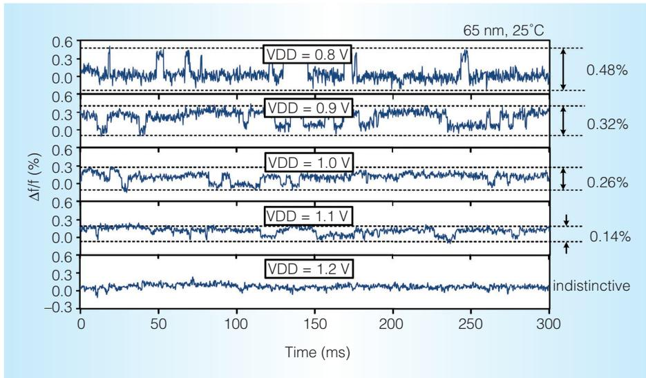
Figure 10. Frequency fluctuation due to RTN at different supply voltages. The amplitude of the frequency shift decreases with increasing  $V_{DD}$ . The capture time (the time in low-frequency states) and the emission time (the time in high-frequency states) have a positive and negative dependence on voltage, respectively.
