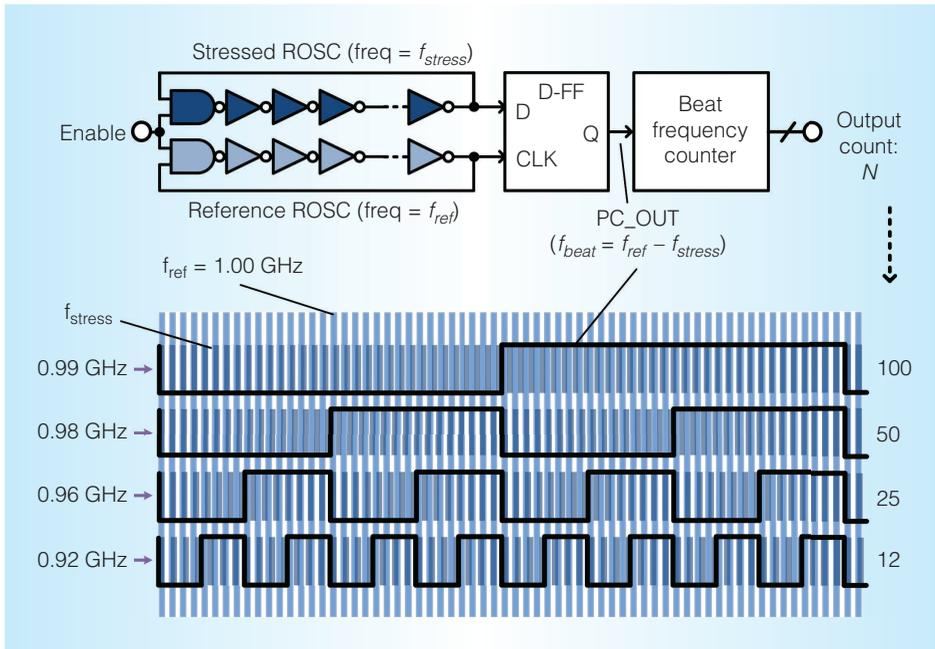
Figure 4. Concept behind the beat frequency detection system. Small frequency shifts induced by circuit aging are magnified by measuring a single ring oscillator's beat frequency (that is,  $\Delta f$ ) rather than its raw frequency.
