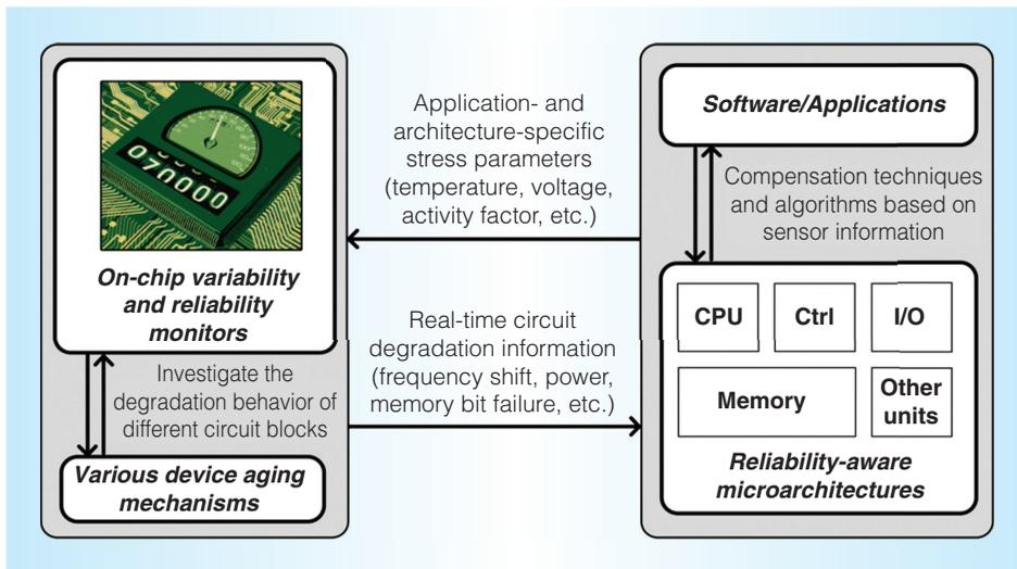
Figure 1. A cross-layer aging-compensation framework based on in situ reliability monitors. On-chip aging sensors provide real-time circuit degradation information that could trigger the compensation of aging at the architecture and application level.
