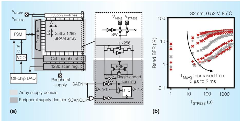
Figure 9. Static RAM (SRAM) odometer for characterizing bit cell failure. Chip diagram (a). Read bit failure rate (BFR) degradation measured using different measurement times (b).
