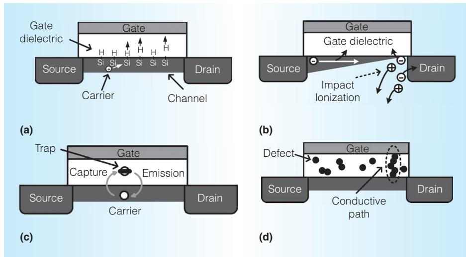
Figure 3. Transistor cross sections illustrating negative-bias temperature instability (NBTI) (a), HCI (b), RTN (c), and TDDDB (d). Positive-bias temperature instability (PBTI) is equivalent to NBTI but occurs in an *n*-channel metal oxide semiconductor (NMOS) device.
