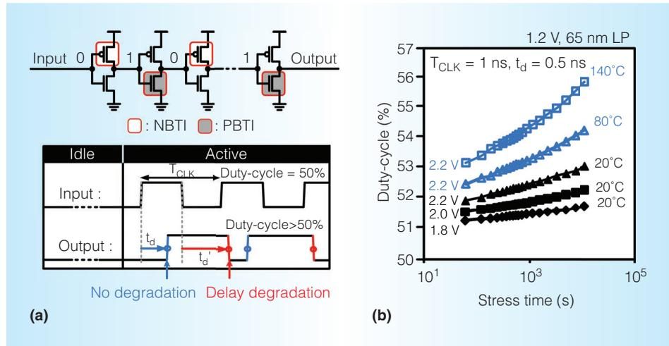
Figure 8. Duty-cycle degradation in a buffer chain due to alternating NBTI and PBTI stress. Asymmetric delay degradation of rising and falling edges results in duty-cycle shifts (a). Duty-cycle shift of a logic path under different stress voltages and temperature (b).
