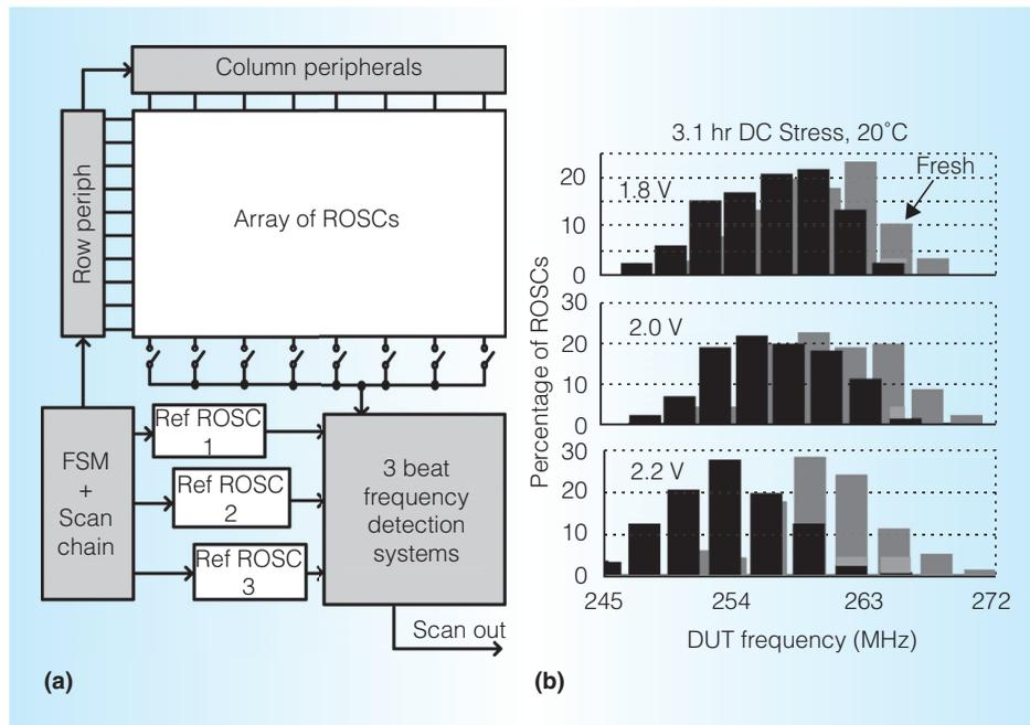
Figure 6. Statistical odometer for understanding aging variability. Top-level system diagram (a). The shift in frequency distributions can be efficiently measured using an array-based circuit (b).
