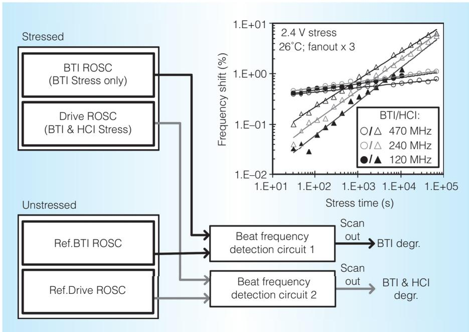
Figure 5. All-in-one odometer system for separately monitoring BTI- and HCI-induced frequency degradation. The inset shows measured data from a 65-nm test chip.
