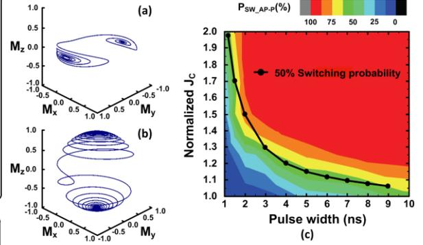
Fig. 2. Model verification results. (a) Dynamic spin motion for IMTJ. (b) Dynamic spin motion for PMTJ. (c) Comparison with experimental data.
