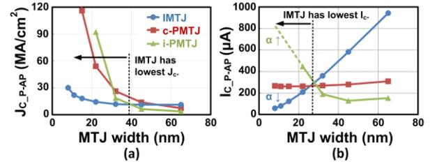
Fig. 3. Scaling trend of (a) critical switching current density and (b) critical switching current for various MTJs. (t<sub>sw</sub>=4ns)
