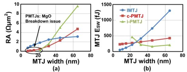
Fig. 4. Scaling trend of (a) RA product and (b) MTJ switching energy for various MTJs based on read/write operation margin.
