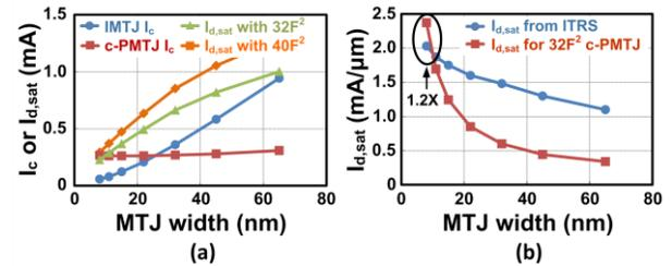
Fig. 6. (a) Bit-cell size for sufficient switching current throughout the MTJ scaling. (b) Drive current required for c-PMTJ to have the same bit-cell size as IMTJ. Higher drive current than ITRS projection is needed at 8nm node.
