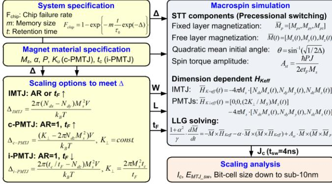
Fig. 1. Scaling analysis using a physics-based MTJ model.
