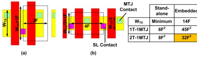
Fig. 5. Comparison of STT-MRAM bit cell layout styles. (a) 1T-1MTJ cell layout for stand-alone applications. (b) 2T-1MTJ cell layout for embedded applications. The W<sub>TX</sub> is adjusted to be a multiple of 2 for 2T-1MTJ case.
