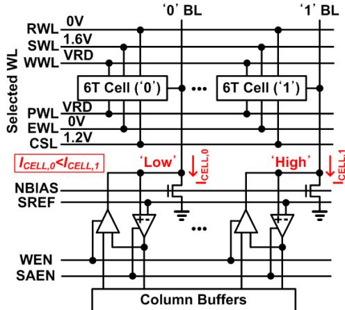
Fig. 5. Read bias condition of the proposed 6T eflash cell.
