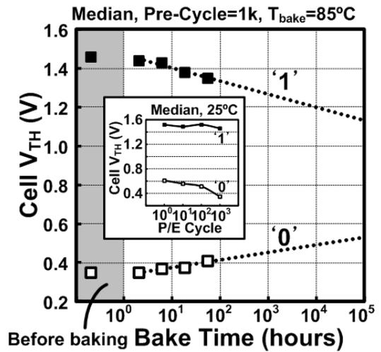
Fig. 11. Measured cell endurance and retention characteristic of the proposed 6T eflash cells.
