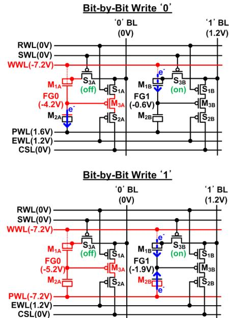
Fig. 4. Bias conditions for bit-by-bit write operations of the proposed 6T eflash cell. '0' BL cell loses electrons from FG during bit-by-bit write '0' operation, while '1' BL cell gains electrons in FG during bit-by-bit write '1' operation.
