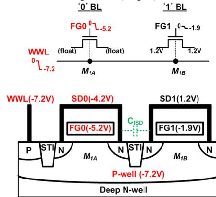
Fig. 3. Selective FG boosting is enabled by the preferential coupling for '0' BL cells where the source and drain node (SD0) of the coupling transistor ( $M_{1A}$ ) is floated, while the corresponding node (SD1) for '1' BL cells is tied to VDD (1.2V). The differently boosted FG voltage levels for '0' and '1' BL's are utilized for the bit-by-bit electron tunneling occurred in the program transistor  $M_{2A}$ ,  $M_{2B}$  (shown in Fig. 4) during write operations.
