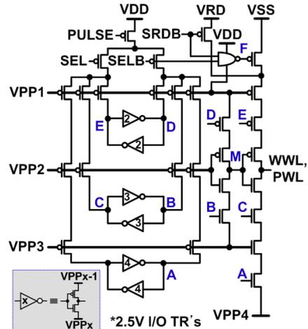
Fig. 8. Multi-story negative HVS implemented in a standard logic process.
