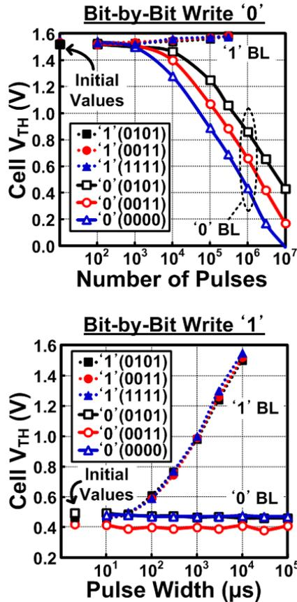
Fig. 10. Measured bit-by-bit write ‘0’/‘1’ phase and disturb results.
