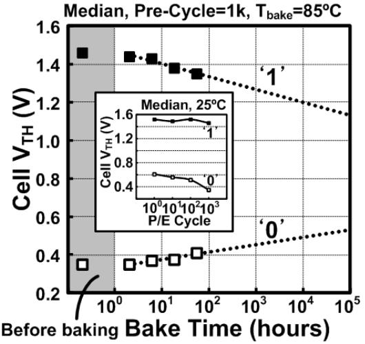
Fig. 11. Measured cell endurance and retention characteristic of the proposed 6T eflash cells.
