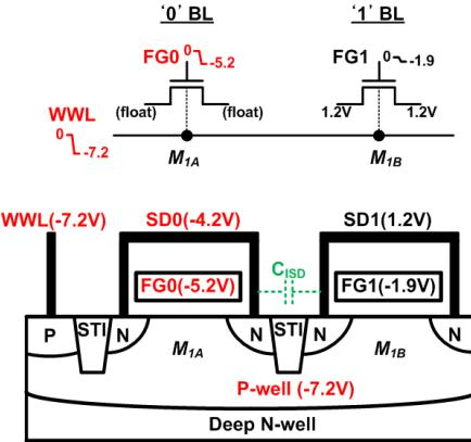
Fig. 3. Selective FG boosting is enabled by the preferential coupling for ‘0’ BL cells where the source and drain node ( $SD0$ ) of the coupling transistor ( $M_{1A}$ ) is floated, while the corresponding node ( $SD1$ ) for ‘1’ BL cells is tied to VDD (1.2V). The differently boosted FG voltage levels for ‘0’ and ‘1’ BL’s are utilized for the bit-by-bit electron tunneling occurred in the program transistor  $M_{2A}$ ,  $M_{2B}$  (shown in Fig. 4) during write operations.
