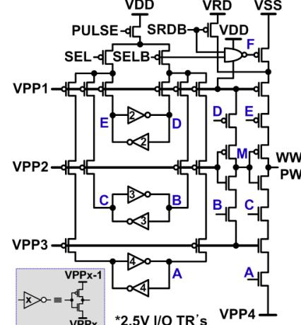
Fig. 8. Multi-story negative HVS implemented in a standard logic process.
