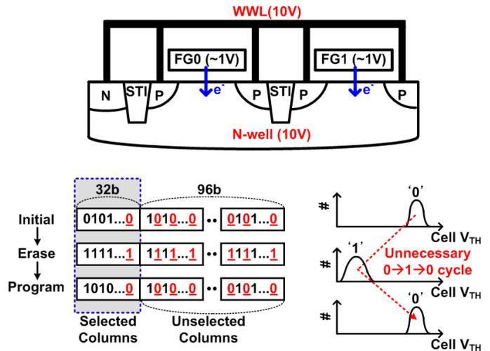
Fig. 1. In prior WL-by-WL erasable eflash memories, high voltage is applied to the tunnel oxide in the entire cells of the selected WL, causing an electron tunneling from the floating gate, which adds an unnecessary erase/program cycle for the unchanged '0' cells in the selected and unselected columns.
