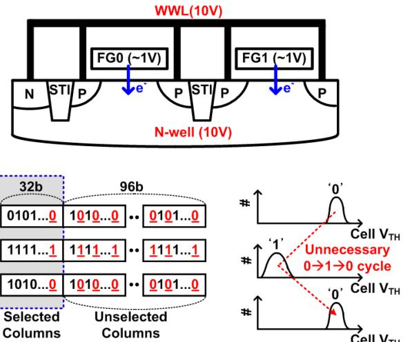
Fig. 1. In prior WL-by-WL erasable eflash memories, high voltage is applied to the tunnel oxide in the entire cells of the selected WL, causing an electron tunneling from the floating gate, which adds an unnecessarily erase/program cycle for the unchanged ‘0’ cells in the selected and unselected columns.
