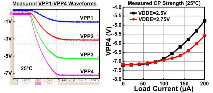
Fig. 7. Measured output characteristic of the voltage doubler based negative charge pump.
