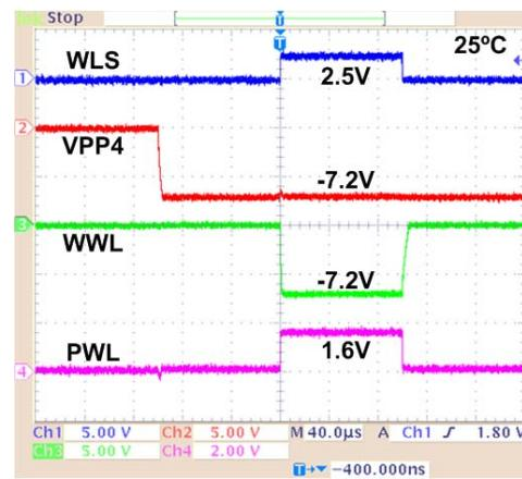
Fig. 9. Measured CP and HVS waveforms for a bit-by-bit write '0' pulse.
