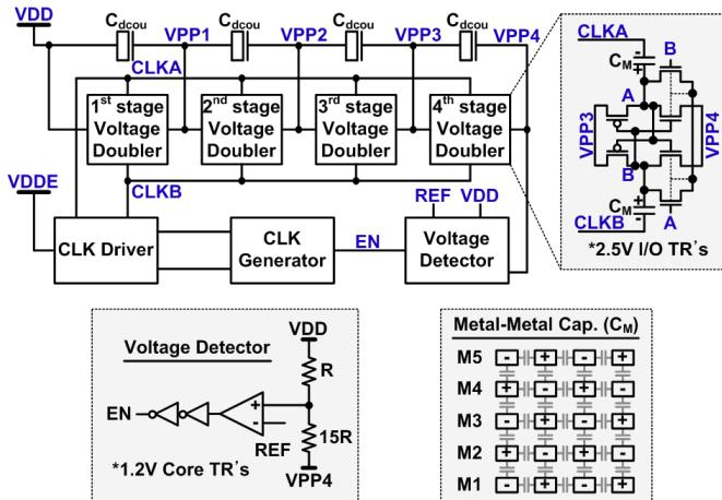
Fig. 6. Voltage doubler based negative charge pump generating VPP1-VPP4 levels is implemented in a 65nm standard logic process.
