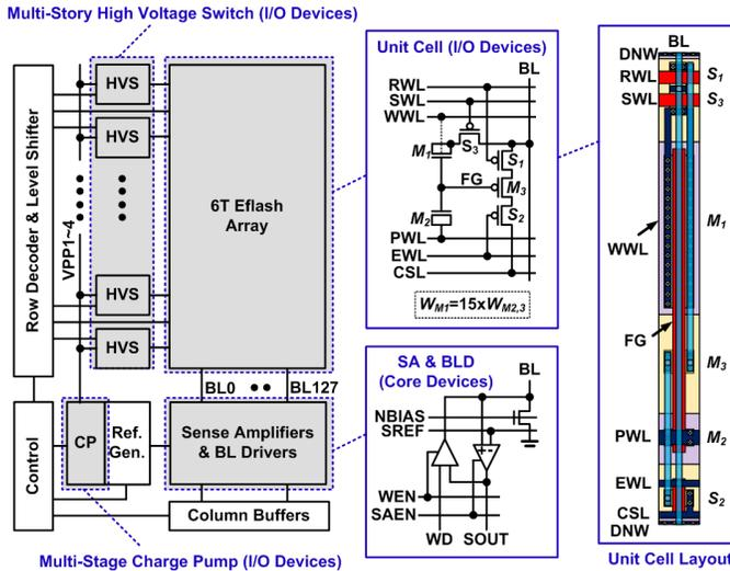
Fig. 2. Proposed bit-by-bit re-writable embedded flash memory including 6T cell array, charge pump, high voltage switch, sense amplifiers & BL drivers was implemented using core and I/O devices in a standard CMOS process.
