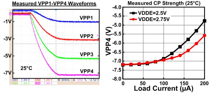
Fig. 7. Measured output characteristic of the voltage doubler based negative charge pump.
