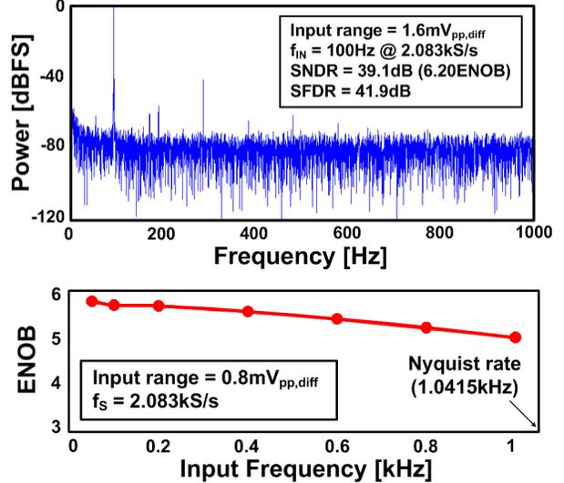
Fig. 10. Measured FFT for a 1.6mV<sub>pp</sub> AC signal with key ADC specifications (upper). ENOB versus input frequency data (lower).
