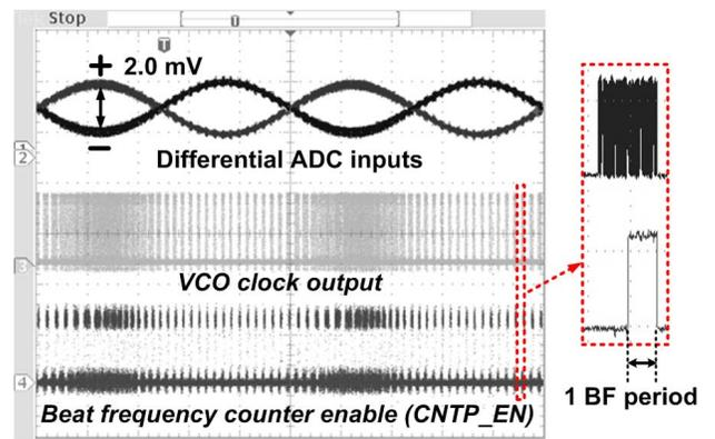
Fig. 5. Waveforms from BF-ADC test chip for a 4 mV<sub>pp</sub> differential input.
