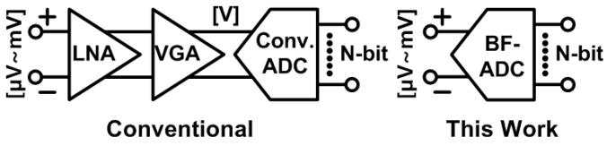
Fig. 1. The focus of this work is on direct acquisition of small input signals without using an LNA or VGA.
