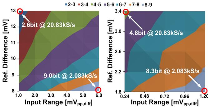
Fig. 7. Measured ADC resolution as a function of input range and reference voltage difference.
