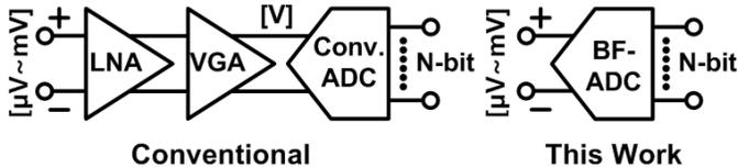
Fig. 1. The focus of this work is on direct acquisition of small input signals without using an LNA or VGA.
