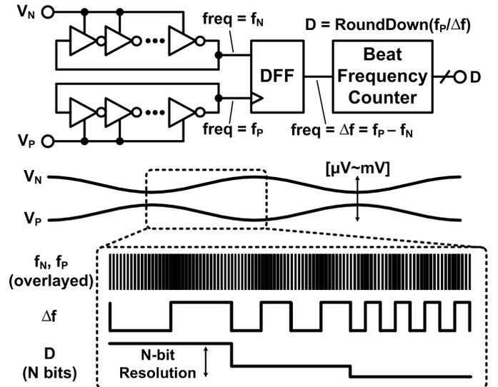
Fig. 2. Operating principle of proposed BF-ADC.
