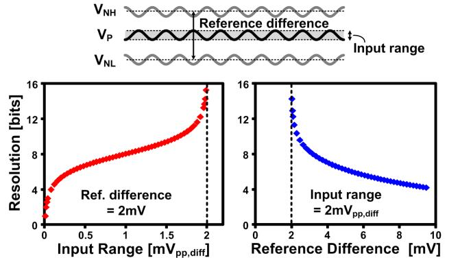
Fig. 6. Simulated resolution as a function of input range and difference between two AC-coupled reference voltages.
