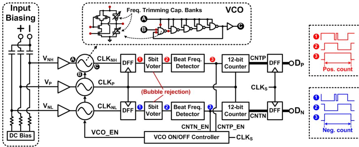
Fig. 3. Dual reference BF-ADC circuit for improved resolution.
