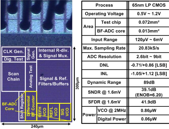
Fig. 12. Chip microphotograph and feature summary table.
