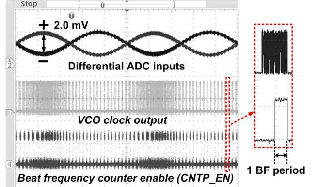
Fig. 5. Waveforms from BF-ADC test chip for a  $4 \text{ mV}_{\text{pp}}$  differential input.
