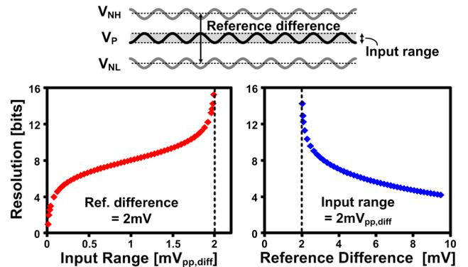
Fig. 6. Simulated resolution as a function of input range and difference between two AC-coupled reference voltages.
