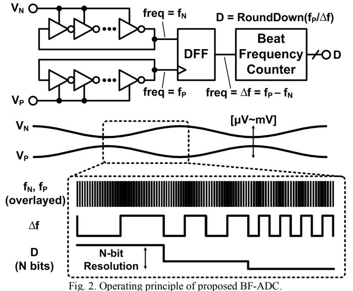
Fig. 2. Operating principle of proposed BF-ADC.
