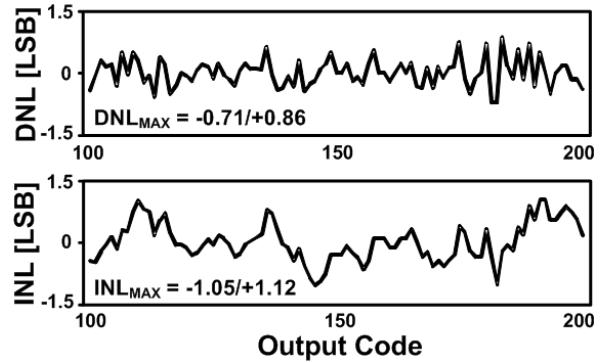
Fig. 9. Normalized DNL and INL from the measured output code.
