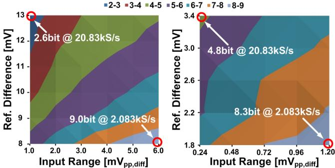
Fig. 7. Measured ADC resolution as a function of input range and reference voltage difference.
