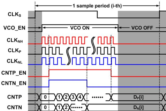
Fig. 4. Timing diagram for one sampling period.
