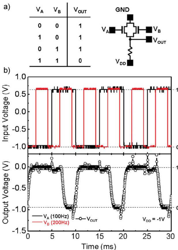
**Figure 5.** NAND logic gate based on printed gel-OTFTs and a printed resistor. The substrate was  $\text{SiO}_2(300 \text{ nm})/\text{Si}$ . a) Logic sequence and circuit diagram. b) Dynamic response of the NAND gate. The red and black lines in the top panel represent two input voltages,  $V_A$  and  $V_B$ , respectively. The open circles in the bottom panel show the output response. Transistor dimensions:  $L = 25 \mu\text{m}$ ,  $W = 500 \mu\text{m}$ .
