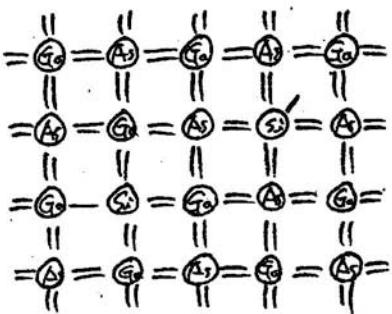
When a Si atom with four Valence electron is inserted into the missing Ga site, there is one extra electron.
